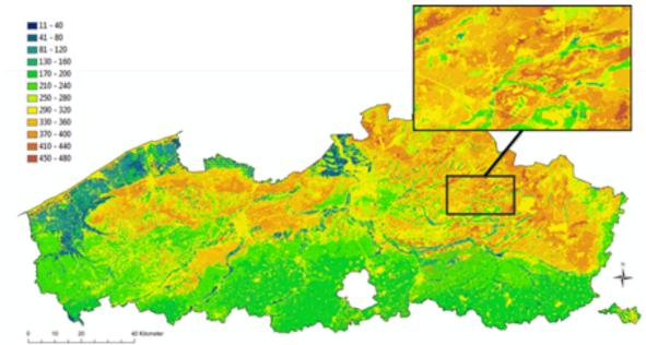
Figure 18. Potential infiltration for the Flemish Region, taking into account soil texture and soil hydrology (Staes and Meire, 2013).
