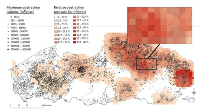
Figure 28. Relative abstraction ratio (percentage of annual recharge abstracted), groundwater abstraction wells (unconfined) and virtual buffers of needed recharge area (8 m<sup>3</sup> of recharge area for each m<sup>3</sup> annually abstracted) (Staes and Meire, 2013).
