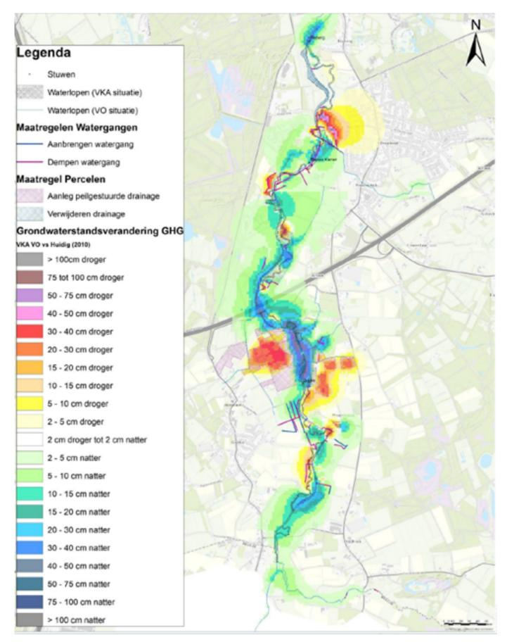
Figure 70. Expected changes in groundwater level (GHG) as result of the measures of the concept design of the project Markdal
