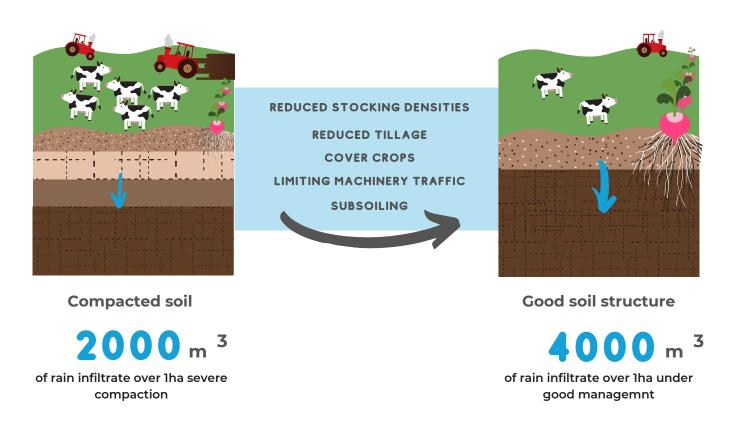
Figure 56. A comparison of compacted and non-compacted agricultural soils and management practices that can remediate soil compaction.
