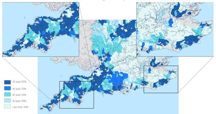
Figure 26. This figure shows how reliable (i.e. the proportion of time that it could be used) a new abstraction license might be based on how much water is available at different flows. The percentages relate to the amount of time that additional water may be withdrawn without harming the environment. Management Strategy (CAMS) 2020).
