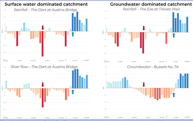
Figure 11. Rainfall and river flow in Runoff dominated catchment (i.e. surface water dominated) vs. rainfall and groundwater in groundwater dominated catchment.
