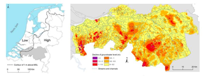
Figure 20. Left: Division of the country in high and low part (Noord-Brabant: grey). Right: Simulated decline in groundwater level due to change in land use between 1950 and 2010.
