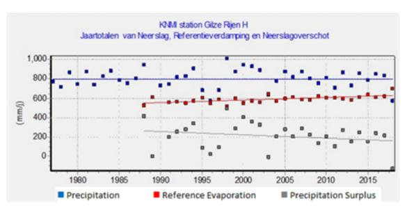
*Figure 45. Yearly precipitation (blue), Reference evaporation (red) and Precipitation surplus (grey) from the weather station Gilze Rijen in Noord-Brabant from 1978 till 2018. Source: KNMI, 2019.*
