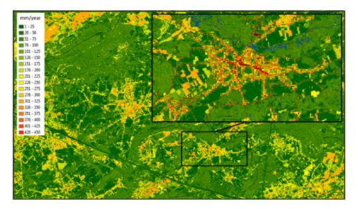
Figure 16 Impact of soil sealing and canopy interception on infiltration (net losses, compared to the potential infiltration) (Staes and Meire, 2013).
