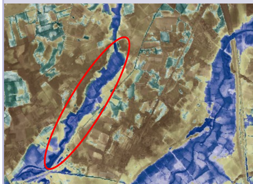
The red oval indicates the part of the Bijloop along which several measures will be implemented. The water system map confirms the potential to restore a natural wetland (with potential for permanently wet areas and temporary wet areas indicated in blue and green).
