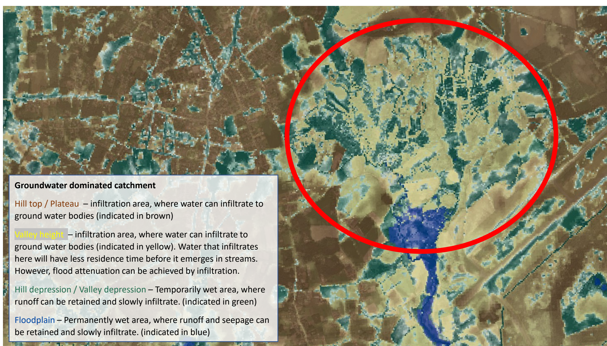
The water system map, applied to the demonstration site. The red circle highlights the larger area of the demonstration site. The green and blue areas highlight locations with a high potential to restore wet nature, such as wet Alder Forest.
